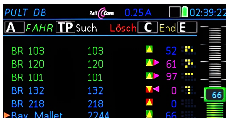
Screenshot (detail) from the MX33 controller: CAB DB (V) with a denser row layout than in the app; selection via scroll wheel, not touch.
