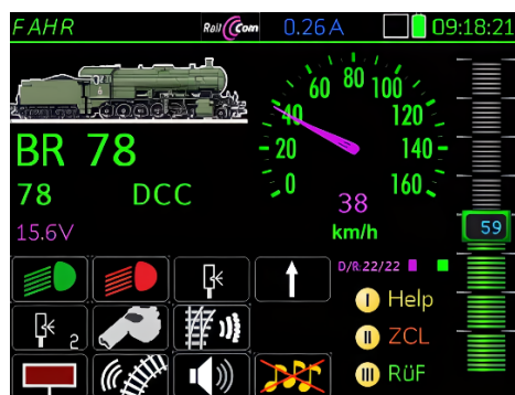
Screenshot of the MX33 controller: full screen view whilst driving
