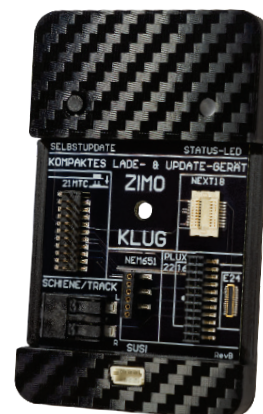
▲ ZIMO KLUG Compact sound loading and decoder update device with integrated interfaces
