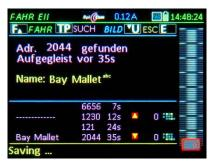
The display-picture of the MX32 shows the results of the track-on search: in this case, the address 2044 was found, which obviously was registered in the MX10 as Bay Mallet; the track-on search nevertheless also works for new addresses. In the field beneath further addresses are listed (mixed: new ones and also known ones), which were "tilted" in the same period of time (1 minute after starting the search).
