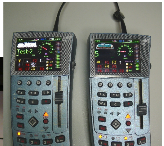
Situation "Broadcast Stop" on the track-1 with touch fields for restarting (ON) or OFF via Power Switch on all cabs.
