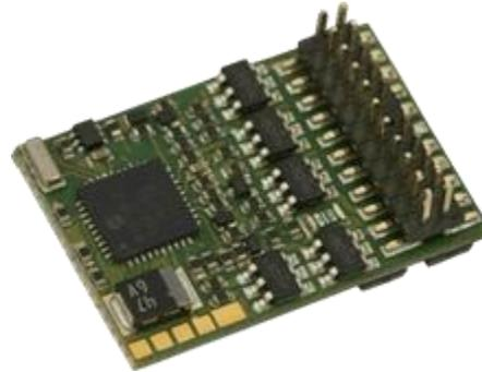
DCC + RailCom, DC-analog, MM, AC-analog
