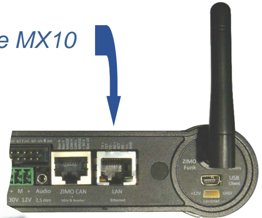
LAN socket on the back of the device
