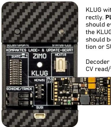
KLUG with decoder connected directly. **Please note:** only one decoder should ever be connected directly to the KLUG; additional decoders should be connected via rail connection or SUSI socket.
