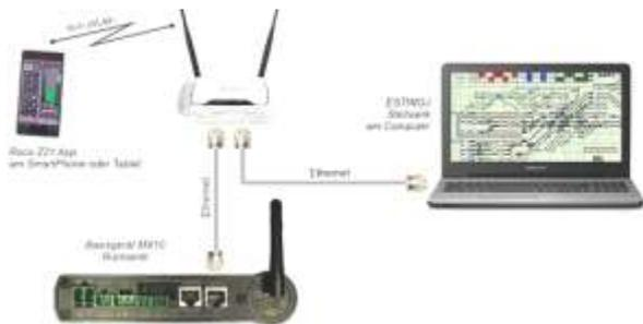
A **static IP-address** must be set (in “properties” of the internet protocol, TCP/IPv4), which fits the preset IP-address of the MX10: **192.168.1.100** (if “100” is already used by another LAN-device, a different value is possible).
