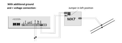
The connection differs from the above diagram when using the "old" ZIMO data format (MX1/MULT, MX1/Z):
