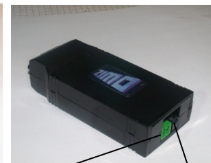
To "update track", to power supply control-LED's behind socket
