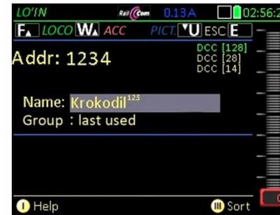
In the window '**LOCO IN**' on the MX32/MX33 controller, a (new) vehicle address is entered and - if desired - given a name. Further GUI elements can also be activated using F-keys (opening in the screen **LOCO**)
