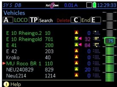
Screen '**SYS DB**' on the controller MX32/MX33 shows the entire system-wide object database **SYS DB** (i.e. all addresses in the digital centre), with the objects available locally in the controller in **blue/green** line colour, and thus indirectly the **LOCO DB**.
