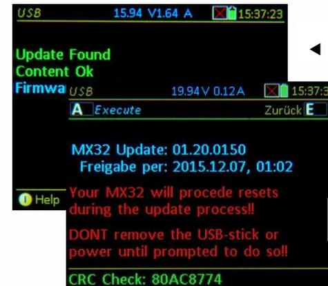
Firmware Check: The MX32 tests the software to be loaded for bad or corrupted data and shows the result. After this presentation, the control panel automatically goes to the update information screen.
