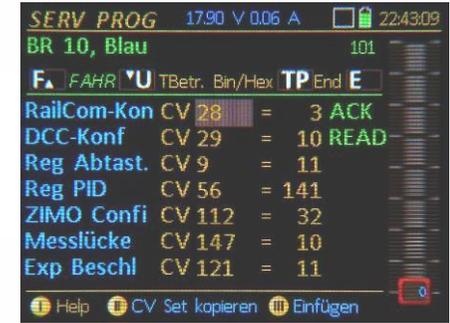
**ATTENTION:** With the "Paste" command the CV-lines are only listed but NOT yet sent to the decoder. This must be carried out afterwards for each individual line; that is, in practice:
