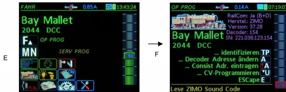
The first screen when entering **OP PROG** is a menu screen; ABOVE is the display shown of a decoder with working **RailCom feedback**, which makes identification possible: Information such as manufacturer, software version and decoder ID are read out and displayed automatically (in magenta, the color for RailCom);
