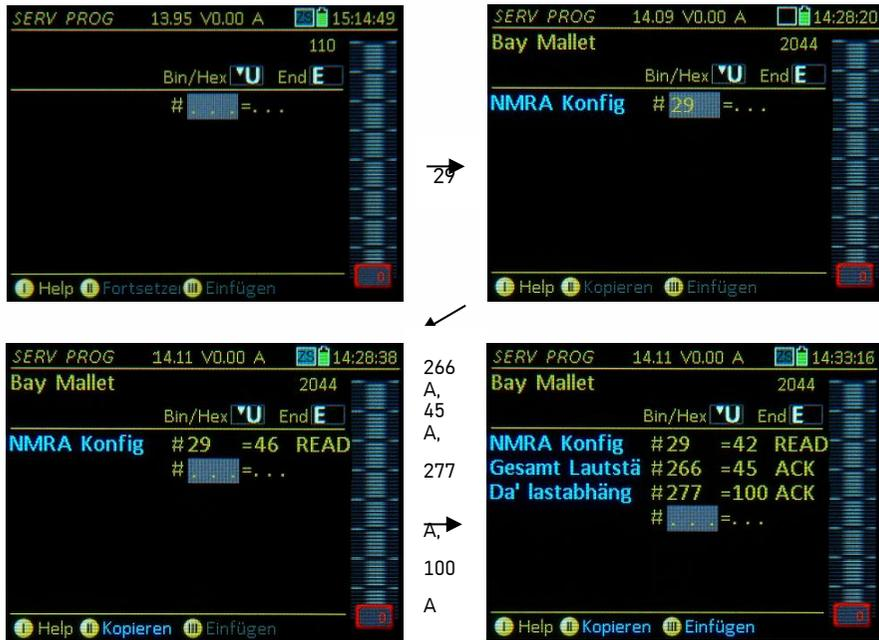
CV programming success (or failure) report at the end of each line after completion with the **A-Key**:
