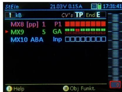
This display therefore shows the elements to be monitored or switched for each module found: in the case of the MX8 the 16 turnouts in two groups (switchable with ↑ (Shift) key), in the case of the MX9 the occupancy statuses of the 16 track sections and the HLU statuses of the 8 main sections (combining two track sections in each case). The turnouts or the HLU states of the track sections can be selected using the number keys.
