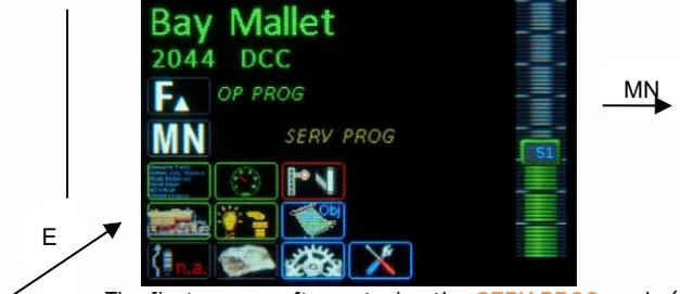
The first screen after entering the **SERV PROG** mode (with E + MN keys) is the programming menu, which also functions as a "security question" to prevent accidental deletion of decoder addresses or data.
