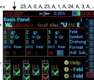
After entering **SWI DEF** the input blocks for the first three fields (turnouts) are displayed, **Scroll wheel** → Continue scrolling through the fields (in the panel AND in input blocks)
