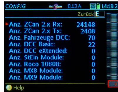
Various current data regarding communication and devices connected to the command station.
