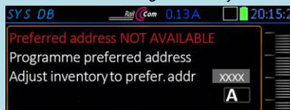
**Login case 2.** ... A partial match entry is found in the system database; with **DID** of the reported decoder, but **different address** (not the desired one).
