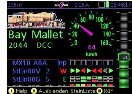
In this example, there are several StEin modules in the list, two of which just show the turnout positions and the other track sections with different HLU and east-west states.
