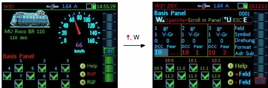
In **SWI DEF**, three input blocks are assigned to three panel fields (i.e. one line of the panel). The number at the top left of the input block shows the field number, i.e. the panel field for which changes are currently being made.
