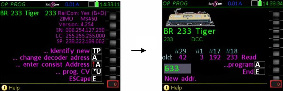
An input field appears under the "Old data", in which ▲ the new address is entered.
