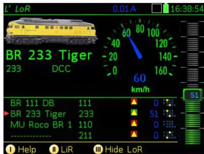
Usually, the **LoR** is displayed in the lower half of the screen, while the upper part is still available for the active vehicle, as well as the side bar.
