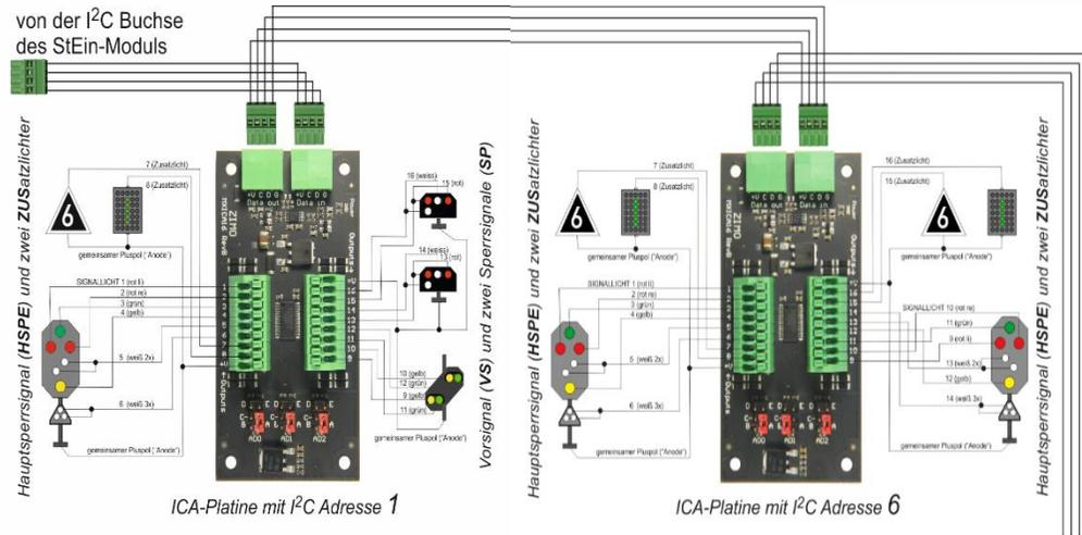
Either all lines can be filled in completely (starting with "Symbol") or only the connection location of the signal can be specified, which is agreed by specifying the "first wire" - this is generally the red light (or the "strongest" stop, e.g. the two yellow lights of a distant signal. The **SWI DEF** lines "Symbol" are optional, the lines "Format" and "Addr Sub" are to be filled in as follows (slightly different from the information on the previous page):
