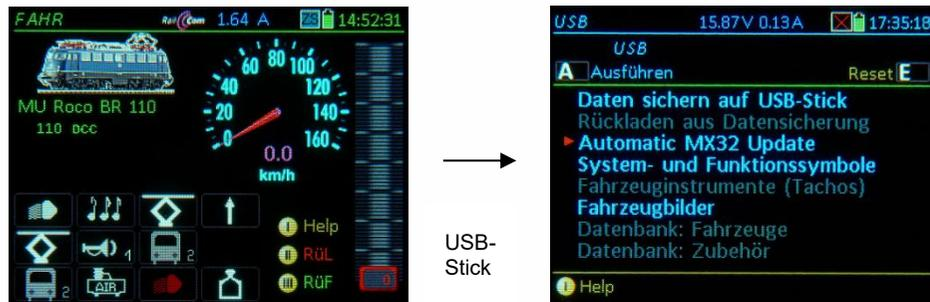
**A-Key** → the "table of contents" is displayed: a list of entries (in order): "DATA BACK UP to flash drive", "Restore Data", "Automatic MX33 Update" and, after that, the names of expected data (not the actual file names), such as data currently present on the stick (blue) as well as expected that is not on the stick (gray) but could be.
