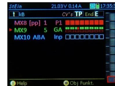
The easiest way to re-address is of course to have only one MX8 or MX9 module connected to the CAN bus in addition to MX10 and MX32/MX33; other CAN bus devices such as control panels are irrelevant in this respect.
