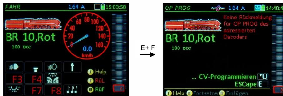
**NOTE: OP PROG** is possible while driving or at standstill. The vehicle can be driven normally while programming or reading out data. Of course, data transmission tends to be worse while driving and it is therefore recommended to drive only when RailCom feedback is available (or the programming changes can be seen instantly by the vehicle's behavior).
