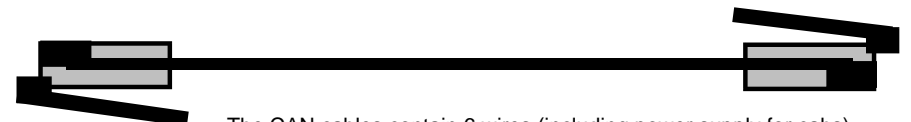
The CAN cables contain 6 wires (including power supply for cabs) and are ended with "telephone" plugs fitting to the sockets in ZIMO devices.
