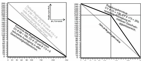
The overall intensity of load compensation can be defined with CV #58 from no compensation (value 0) to full compensation (value 255). Useful values range from 100 to 200.
