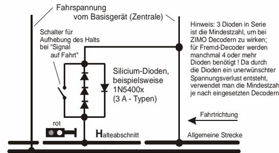
The different voltage drops across the diodes results in an asymmetry of about 1 to 2 V. The direction in which the diodes are mounted determines the polarity of the asymmetry and with it the driving direction a signal stop is initiated.
