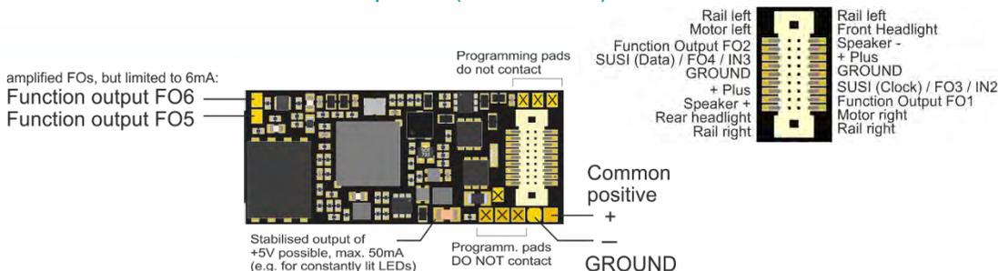
Bottom side (with optional external extension of the stay-alive capacitor)
