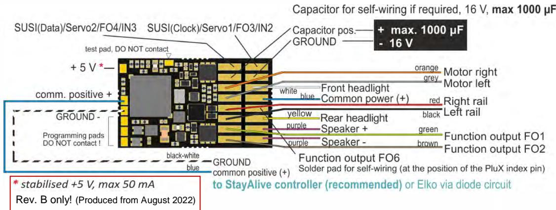
External capacitors **directly on miniature decoders MS480, MS490, MS500**
