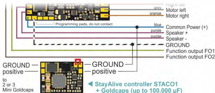
Schematics MS500, MS500R, MS500F Top side with wires
