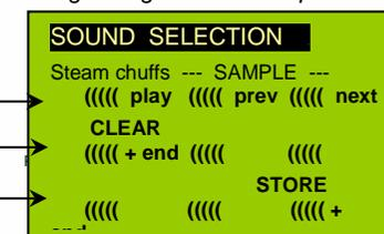
**F0** = play: plays back the current chuff sound for evaluation; only possible with the engine at a standstill; the chuff sounds are played back automatically when the engine is moving.
