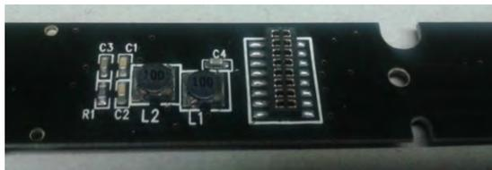
**Remedy:** The "harmful" capacitor on the PIKO locomotive circuit board is usually marked "C4" and must be removed. Normally, the locomotive circuit board has to be removed for this, because the capacitor is fitted on the underside.
