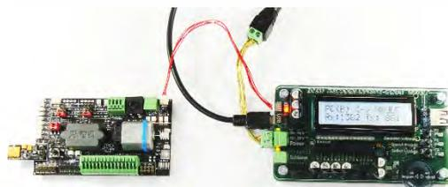
a "Next18" decoder for SW update and sound loading to MSTAPK; connection to MXULFA via "SUSI" cable. NO cable "rail"! Software and sound projects from computer (programs ZSP or ZCS) via USB cable.
