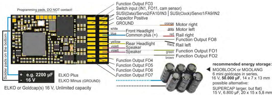
Schematics MS450, MS450R, MS450F Bottom side with wires
