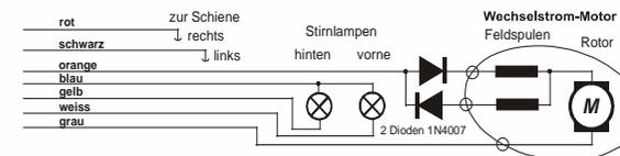
Most locomotives with AC motors get the power supplied by a third rail, which is of no significance as far as the motor hook-up is concerned. The above schematic is therefore valid for AC locomotives running on two or three rail track (instead of "right rail" and "left rail" think "outside rails" and "center rail").
