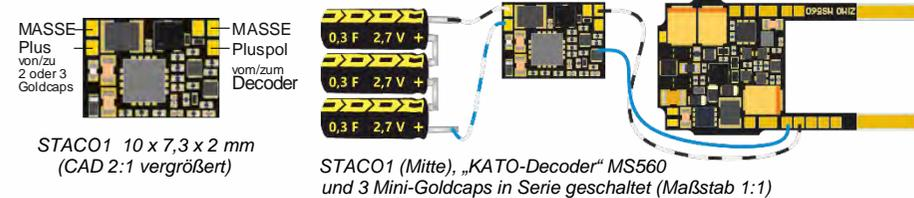
The StayAlive controller is connected to the terminals (solder pads or wires) "Common positive" and "GROUND" of the decoder (two-pole!).
