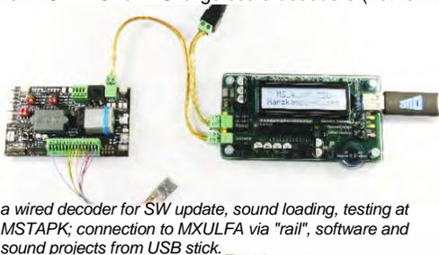
a wired decoder for SW update, sound loading, testing at MSTAPK; connection to MXULFA via "rail", software and sound projects from USB stick.
