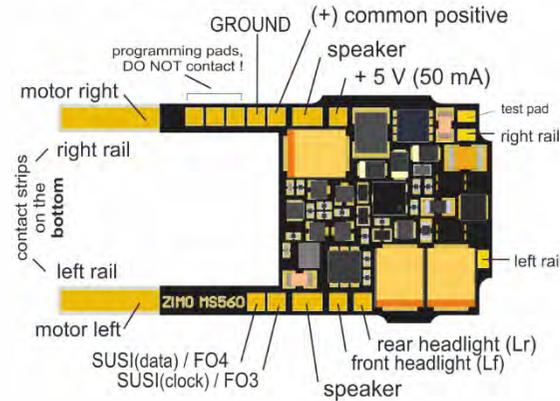
In addition to the actual (main) decoder - in this case the MS560 sound decoder - **the equipment of KATO vehicles** (mostly multiple unit express trains such as ICE-4 or Shinkansen) includes special function decoders for the headlights and interior lighting.
