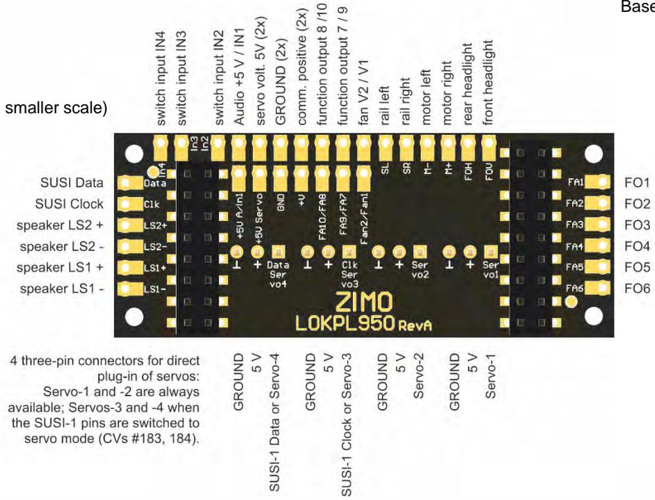
4 three-pin connectors for direct plug-in of servos: Servo-1 and -2 are always available; Servos-3 and -4 when the SUSI-1 pins are switched to servo mode (CVs #183, 184).
