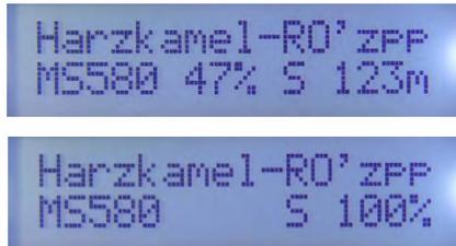
\*) If there are several .zsu or .zpp files on the stick (or both types mixed), the first two files are displayed immediately and the others can be made visible by scrolling. The file marked with an arrow is then ready to be loaded into the decoder. The process is started by pressing key 1 or key 2; the key must match the selected file, i.e. key 1 if the .zsu file is selected (decoder update), or key 2 if the .zpp file is selected (sound loading).
