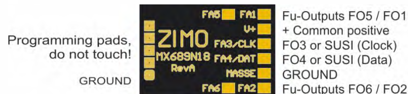
Connection diagram MX689N18 Bottom Side View (Next-18)
