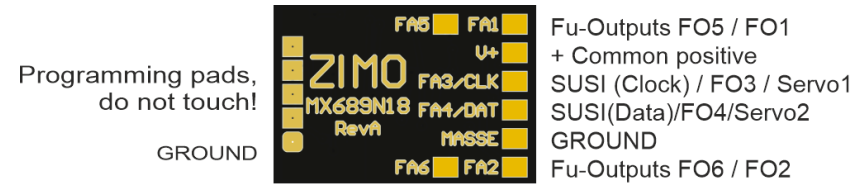
Connection diagram MX689N18 Bottom Side View (Next-18)
