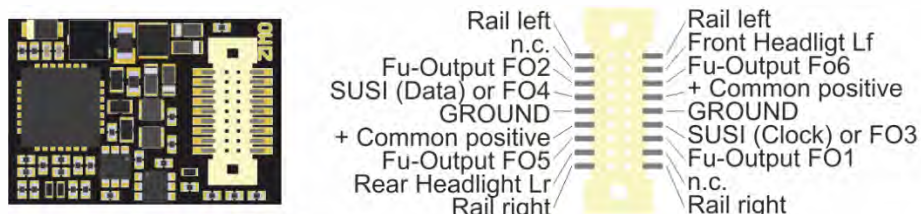
Connection diagram MX689N18 Plug Side View (Next-18)
