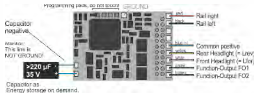
Connection diagram MX686D (bis 2012) Bottom Side (Based on MX631-Series)
