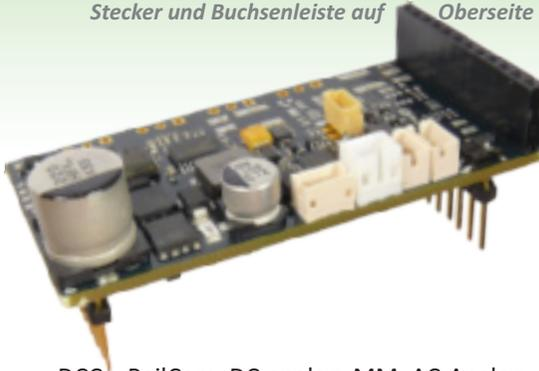
DCC + RailCom, DC-analog, MM, AC-Analog
