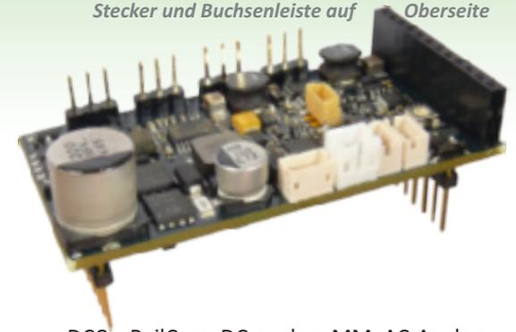
DCC + RailCom, DC-analog, MM, AC-Analog
