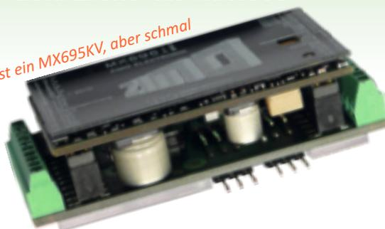
DCC + RailCom, DC-analog, MM, AC-Analog
