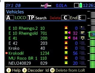
By **activating it** (using the **A** button from the **SYS DB**, grey line), the screen **LOCO** is opened for the address, and it is also entered into the **CAB DB** and **LoR** i.e. **green** line in the screen '**SYS DB**'
