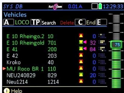
Screen '**SYS DB**' on the controller MX32/MX33 shows the entire system-wide object database **SYS DB** (i.e. all addresses in the digital centre), with the objects available locally in the controller in **blue/green** line colour, and thus indirectly the **CAB DB**.
