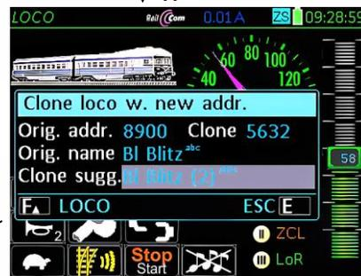
In the 'Clone loco w new addr.' window, the source address is predefined (i.e. that of the active vehicle), while the **clone address** is entered manually. Any address conflicts ('... already exists') are indicated. The name of the clone can either be accepted as suggested ('... (2)') or changed (C key - extend, further C keys - delete character by character, new text).
