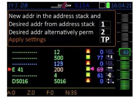
The **system-wide object database** in the '**SYS DB**' window (after E + 6), i.e. the vehicles already known in the system: all entries in your own device (**CAB DB**: **green, blue, turquoise** lines), as well as all those that only occur in the command station (**SYS DB**: **grey** lines).
