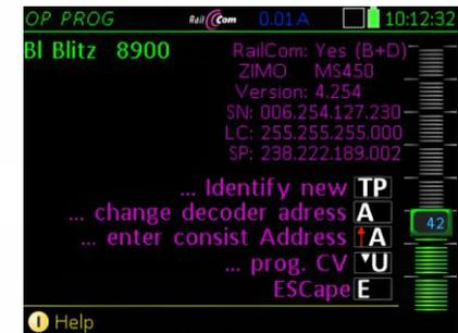
The first screen when entering **OP PROG** is a menu screen; ABOVE is the display shown of a decoder with working **RailCom feedback**, which makes identification possible: Information such as manufacturer, software version and decoder ID are read out and displayed automatically (in magenta, the color for RailCom);
