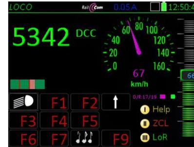
After approx. 0.2 seconds (with undisturbed transmission, otherwise slower), the first data has already arrived: Information for image, selected speedometer disc and name; however, the function icons are still missing, which - depending on the number - account for the majority of the data volume to be transmitted.
