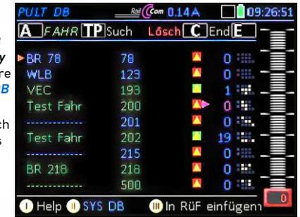
The **SYS DB** and **CAB DB** contain more data than the normal view. Therefore, you can switch between levels: **X-key** or **↑(Shift)** → Switch between pages. 'Normal', ... with track sections', 'with DID'; DID is inserted during RCN-218 registration.
