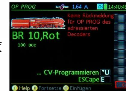
**NOTE: OP PROG** is possible while driving or at standstill. The vehicle can be driven normally while programming or reading out data. Of course, data transmission tends to be worse while driving and it is therefore recommended to drive only when RailCom feedback is available (or the programming changes can be seen instantly by the vehicle's behavior).
