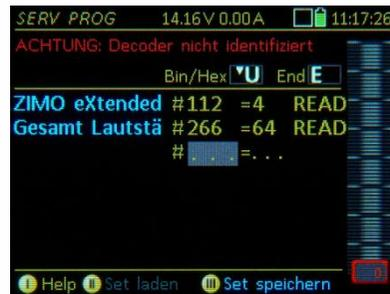
An active shunting mode (R-key engaged) is automatically terminated when calling the CV-programming screen (OP PROG and SERV PROG)!
