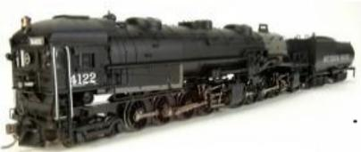
Southern Pacific Railroad's AC-5 class of steam locomotives was the railroad's second class of 4-8-8-2 cab forward locomotives. They were built between July and September 1929 and placed in service soon after construction.
