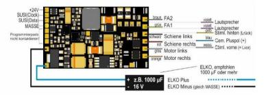
allowed in-rush current, using the full capacity and in most cases it allows the usage of capacitors with a dielectric strength of only 15V (therefore they do not need much space).
