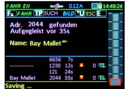
*The display-picture of the MX32 shows the results of the track-on search: in this case, the address 2044 was found, which obviously was registered in the MX10 as Bay Mallet; the track-on search nevertheless also works for new addresses. In the field beneath further addresses are listed (mixed: new ones and also known ones), which were „tilted“ in the same period of time (1 minute after starting the search).*
