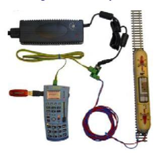
Since October 2008, it has bee possible to load and update decoder software using the MX31ZL and a USB stick. Now it is also possible to load "Ready-to-Use" Sound Projects in the simplest way possible, without using the ZIMO Sound Programmer (ZSP), or a computer. The ZIMO Sound Database contains Sound Projects in two formats ready for download :-
