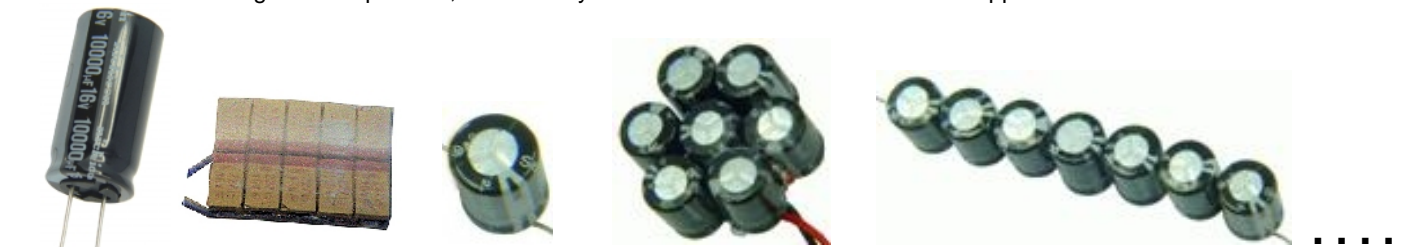
Elko 10000 uF Tantal Packet 5000 uF Goldcap 1F – 2.5 V Goldcap Module with 7 Goldcaps (7 x 1F in series, 0.14 F – 17.5 V)
