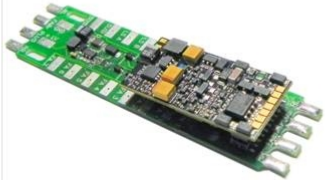
In Photo: ADAPUS15 with 1,5 V low voltage output, 71 x 18 x 4 mm) ADAPUS15 with ZIMO Sound-Decoder MX645P22 plugged in
