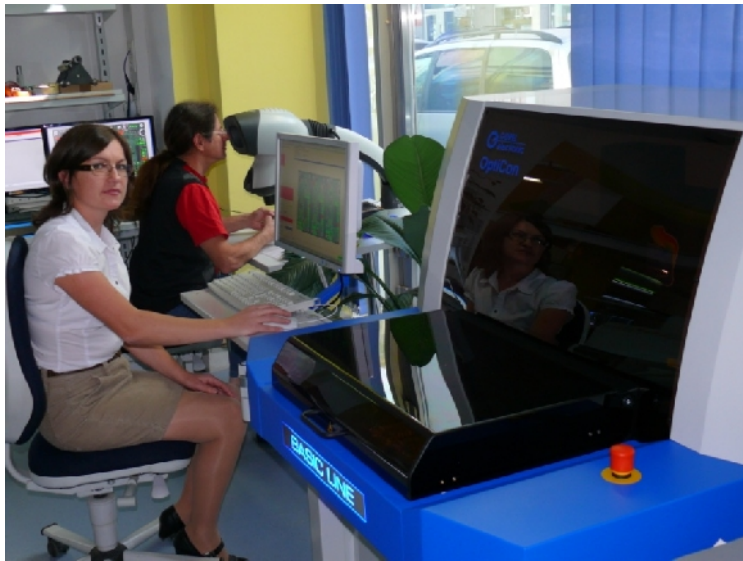
AOI system (while reviewing and checking MXULF boards)
