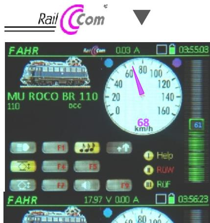
With the help of RailCom the real speed is measured by the decoder and displayed on the speedometer; and, on the speed, the actual speed is displayed in the colour magenta.
