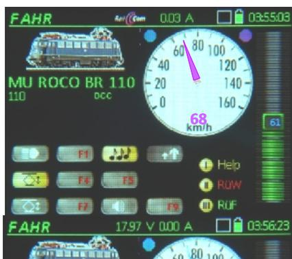
With the help of RailCom the real speed is measured by the decoder and displayed on the speedometer; and, on the speed, the actual speed is displayed in the colour magenta.
