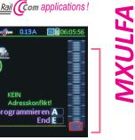
The decoder update and sound loading device loads the new software or sound project either from the USB stick or from the computer, via the track or (the sound) via the SUSI interface (especially fast).
