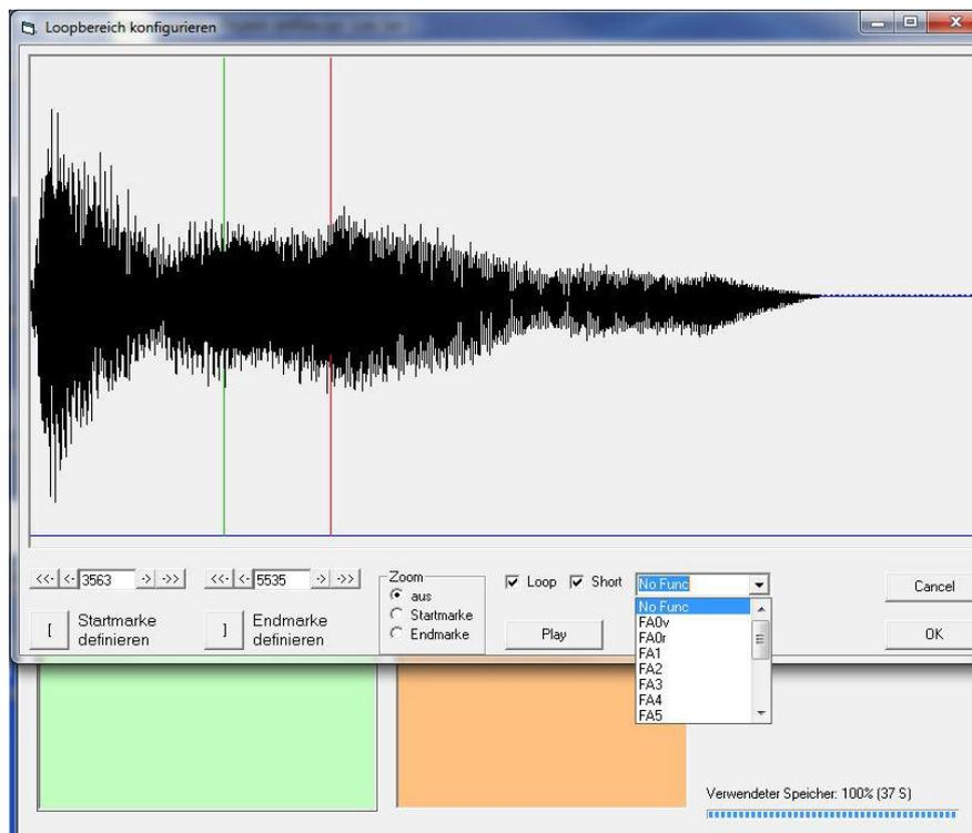
In the selection box is usually "No. func" an output can be selected which always switched on if this sound is currently playing. For example, this can be used to control a red led in the Firebox always when the coal shoveling sound is played.
