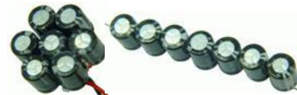
Coldcap module with 7 goldcaps (7 x 1 in series for a total of 140000uf – 17.5V)
