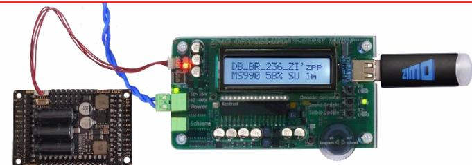
**Simultaneous sound loading** of several MS450 decoders via "SUSI": each decoder must be connected to its own decoder test and connection board MSTAPK2. The **connection boards** can be connected in parallel.
