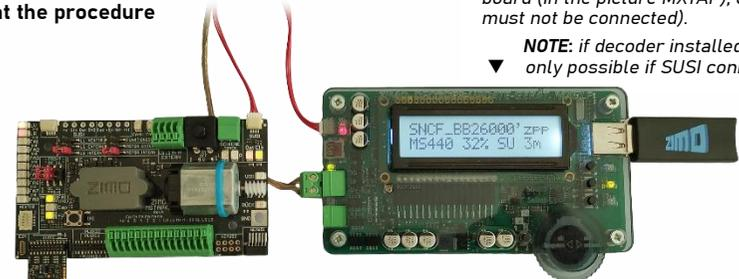
When **100%** is reached: remove the vehicle from the rail, and - if desired - connect/set up **other decoder**, (To avoid a short circuit if the decoder is plugged in incorrectly, it is recommended to disconnect the rail connection using the ON/OFF button on the MSTAP/MXTAP) press **R-Key**
