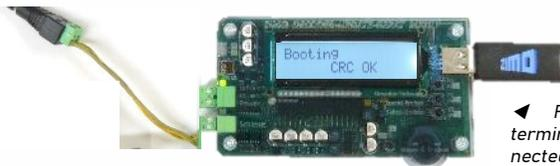
For the self-update, only the power supply (at terminal "Power" of the MXULF) must be connected, and a USB stick with the correct files for the update must be inserted.
