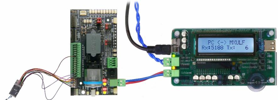
**Note:** MS large scale decoders can also sound load via SUSI, either via MSTAPG or directly connected to the decoder. It is also possible to load another large scale decoder of the same type, connected directly to the second SUSI connection of the MSTAPG. Here in the application example: MS990 on its own SUSI connection directly on the MXULF:
