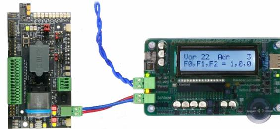
MSTAPK2 with MS480R decoder (8-pin NEM652 interface, loudspeaker not on interface, therefore wires on terminals), connected to MXULF:
