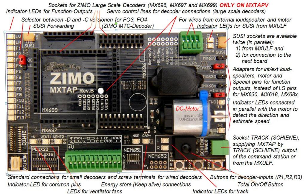
Connections between the *MXTAPV* and the *MXULF*: a 2-pole cable to connect the “Schiene”-plug (track; connectors are supplied with the device) and a 4-pole *SUSI* cable (supplies; *SUSIKAB*).
