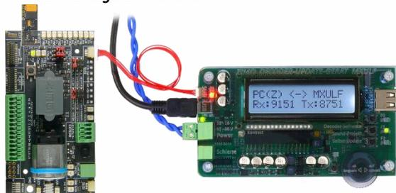
MSTAPK2 with MS590 decoder (Next18), connected to MXULF:
