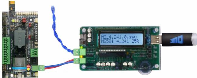
MSTAPG with attached MS950 large railway sound decoder, MXULF connected via rail: sound loading has just been started on the MXULF, the sound project comes from the USB stick.
