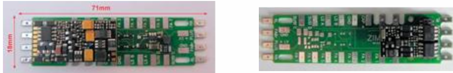
Comparison of an original loco board (left) and the ADAPUS (right)
