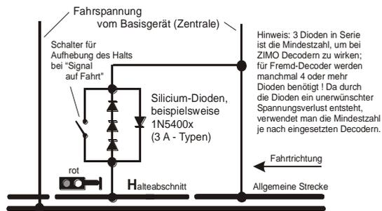
Usually, the stop section contains 3 to 5 silicon diodes in series and one diode in parallel in the opposite direction is the usual arrangement. The different voltage drops across the diodes results in an asymmetry of about 1 to 2V. The direction in which the diodes are mounted determines the polarity of the asymmetry and with it the driving direction a signal stop is initiated.
