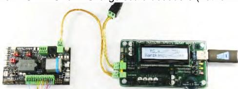
a wired decoder for SW update, sound loading, testing at MSTAPK; connection to MXULFA via "rail", software and sound projects from USB stick.
