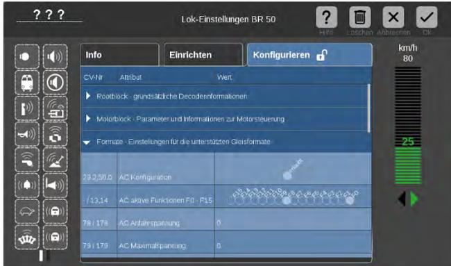
For example: in "Formats" you can configure the AC-analog operation.
