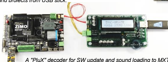
A "PluX" decoder for SW update and sound loading to MXTAPV; connection to MXULFA via "SUSI" cable, but NO cable "rail" from MXULFA to TAP!
