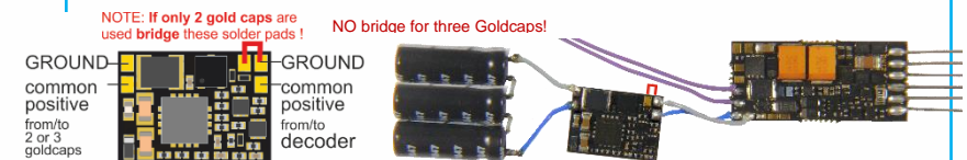
STACO1 10 x 7.3 x 2 mm (CAD enlarged) STACO1 (centre) connected to miniature sound decoder MS490N and 3 miniature Goldcaps in series (scale 1:1)
