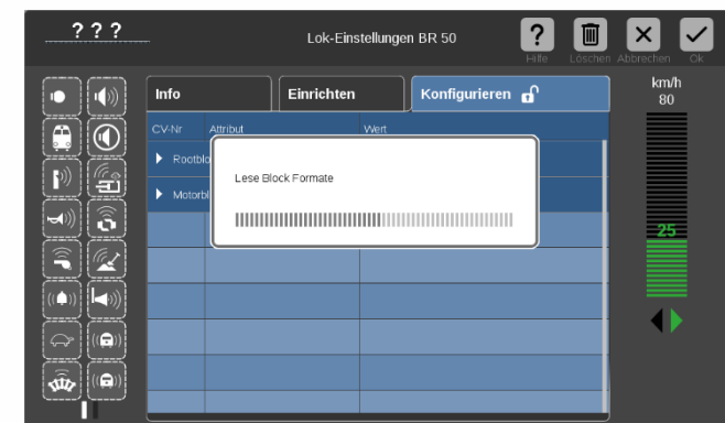
... the "blocks" (i.e. groups of configurations) are read out and opened by the decoder (root block, motor block, formats, sounds, ...).
