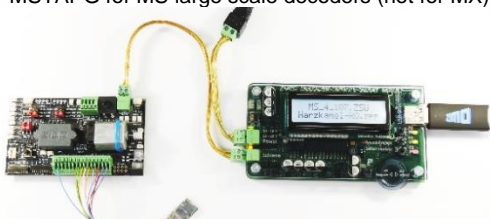
a wired decoder for SW update, sound loading, testing at MSTAPK; connection to MXULFA via "rail", software and sound projects from USB stick.
