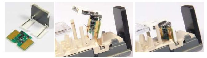
The ZIMO Decoder MX605FL is placed on the decoder holder. Both are then pushed between the contact plates and the plastic holder until the decoder holder engages in the car interior.
