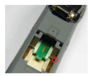
The ZIMO Decoder MX605SL is inserted into the shaft with tweezers. It comes to rest between the contact plates. Make sure that the decoder is pushed to the front oft he shaft.
