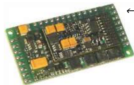
← ADAMTC50 with MX644C plugged in results in a sound decoder with 1.8 A motor (total current) 8 function outputs 2 logic-level outputs (servos, SUSI)– low voltage output 3 Watt audio, 4 – 8 Ohm, 32 Mbit with direct connection for 16 V catalytic capacitors or super caps to 6800 µF Dimensions: 44 x 26.5 x 6 mm
