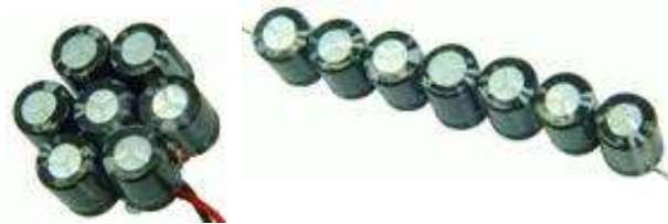
Gold cap module with 7 gold caps (7 x 1F in series = 140000 F - 17.5)
