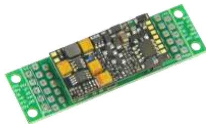
← ADAPLU with MX645P22 plugged in results in a sound decoder with 1.8 A motor (total current) 9 function outputs 2 logic-level outputs (for servos, SUSI) 3 Watt audio, 4 – 8 Ohm, 32 Mbit with direct connection for 16 V catalytic capacitors or super caps to 6800 µF Dimensions: 45 x 15 x 8 mm
