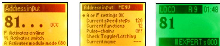
Note: If the mode indicator shows "FAHR" the cab is set for German language. Go to the cab menu by hitting the little round "M" key three times. Use the scroll wheel and scroll down to the line "Auswahl SPRACHE" and hit the "A" key. Scroll down to "English" and hit the "A" key. Hit the "E" key 4 times to get back to the previous screen.
