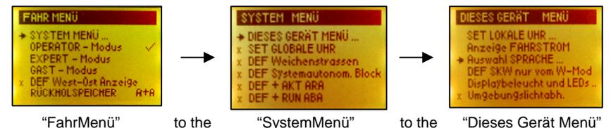
In the "Dieses Gerät" menu, use the scroll wheel on the side and scroll down to "Auswahl SPRACHE"; Accept with the "A" key.
