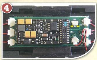
Alternatively, speaker wires can be soldered directly to the decoder, at the blue arrowed solder pads, or to the base of the PCB speaker connector, arrowed yellow.
