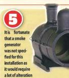
With the retaining screw removed I slid the boiler forwards to disengage its rear location with the main body, taking care not to distort the andrails, then lifted the front end to clear the vacuum pipe fittings.
