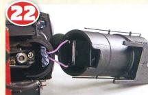
The speaker wires were shortened to the correct length and soldered to the speaker terminals. I used some Blu Tack to hold the wires to the top of the boiler, out of the way of the exposed gears.
