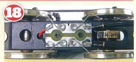
These wires pass through the chassis and are connected to the track pick ups. I de-soldered these and discarded the removed wires. I attached in their place the same coloured wires from the decoder, cut to the correct length to avoid any slack.
