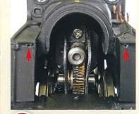
Although tempted to drill out the chimney for sound to escape, careful measuring showed that it would not break out into free space inside the smokebox, which is almost entirely filled with cast resin. Note the 'free' ends of the handrails.
