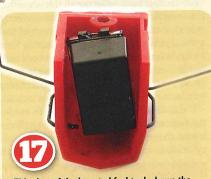
This shot of the inverted fuel tank shows the 8mm x 12mm small sugar cube speaker loosely fitted. For the future, there will be enough space left over to fit LED lighting if required.
