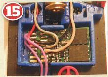
I removed all the unnecessary wires from the decoder and soldered the track and motor wires direct to the decoder, all with the aim of saving space. You can avoid this by joining the wires from the decoder to those of the model; there will be sufficient space to accommodate the insulated joints.
