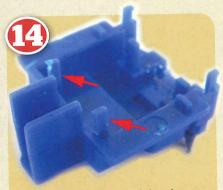
The two rear lugs, arrowed, clip into the enclosure and would interfere with the MX648. They need to be shortened so that they protrude only about 3mm into the enclosure.
