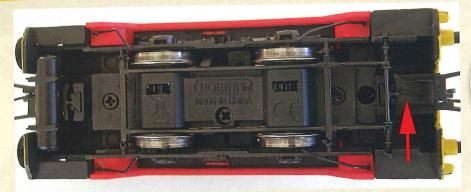
In this general underside view the partly visible gears show that each axle is driven. The screw retaining the cab can be seen, but the NEM coupling, arrowed, must first be removed to reveal the screw holding the fuel tank in place.
