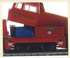
The fuel tank must be released before the main part of the body can be lifted clear by tilting forward as shown here.
