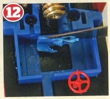
For a snug fit the guard protecting the gears and the rear wall of the enclosure must be trimmed to about half their normal thickness. I used a scalpel for this.
