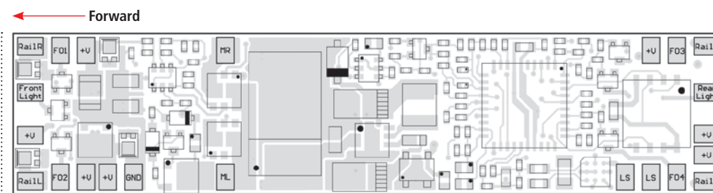
2 Circuit board layout. Bryan Vianco, owner of Streamlined Backshop, designed the MX660 decoder layout with lots of solder pads, including a positive voltage pad adjacent to each function connection, as shown in this diagram.
