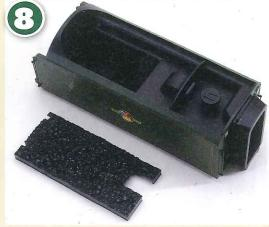
To make space for all this in the tender body, the coal space needs to be cut away from underneath the removable plastic load. Handily, the plastic load can be used to conceal the opening once it has been made.
