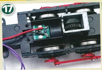
The red and black pick-up wires from the decoder were cut down 45mm in length then soldered to the pick-up tabs on the chassis after baring and tinning their ends.
