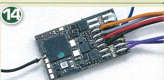
We cut away all the spare wires (yellow, white, green, blue and brown) to reduce the amount of space needed for the chip. We have also now soldered the stay-alive connections to the decoder with the blue positive wire going to the fourth tab down on the right and the black negative wire going to the GND terminal on the left. Adding these wires direct to the decoder must be done very carefully to avoid overheating the chip.
