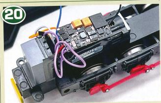
The top of the motor has been wrapped with insulation tape to allow the decoder to be positioned on top. It is held in place with Black Tack. The speaker has been superglued to the chassis and the wires will now tuck between the motor and speaker on reassembly.
