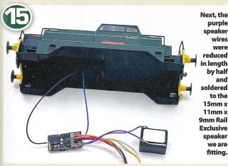
purple speaker wires were reduced in length by half and soldered to the 15mm x 11mm x 9mm Rail **Exclusive** speaker we are fitting.
