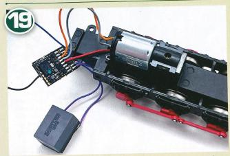
The motor has now been refitted using all its original hardware. Take care to ensure the motor is seated correctly and that the gearbox cover has been fitted the correct way round – if it isn't, it won't fit.
