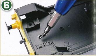
Our first port of call is to install the stay-alive in the rear housing behind the cab. This is held in place with a small crosshead screw – the rearmost of the three under the body.
