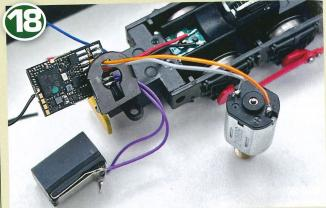
The suppression capacitor has been removed from the motor as the decoder has circuits to do the same job and the orange and grey motor wires have now been connected to the connection tabs on the motor after threading them through its front mount.
