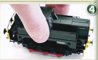
Once the securing screws have been removed, the body lifts straight up from the chassis to reveal the internal workings. Keep the screws safe for reassembly.
