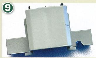
To allow the stay-alive wires to reach the front engine compartment we cut a notch into the bottom of the cab control desk - it's not the neatest, but it won't be seen from the outside.
