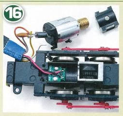
Space saving is important in this model, so we opted for soldering the decoder track and motor connections direct to the model. This involves removing the motor by releasing the two front securing screws and unclipping the rear plastic cover over the gearbox.
