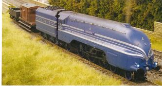
in the tender and the smoke generator and working lamps on the locomotive. The smoke generator is filled via an opening in the top of the boiler backhead in the cab using a pipette and, as we said, with nothing more exotic than bottled water. The filling process is straightforward and requires the locomotive to be tilted forward for access and the addition of two pipettes of water. The right type of pipette is supplied with the model making
