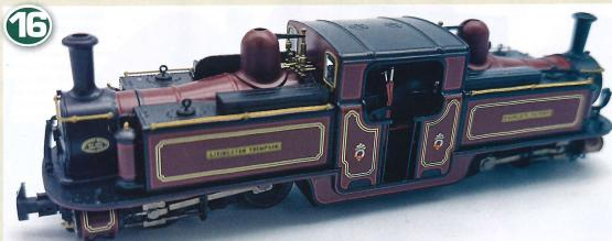
Screw your cover plate back in place and the Double Fairlie is ready for service. Do check your pickups as well - just because you have added a stay alive, this does not guarantee that the locomotive will perform well. It is not going to help if the stay alive can't get the power it needs for a charge to start with.
