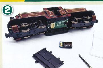
With the cover removed, you now have access to the decoder blank or in this case a DCC decoder which was fitted to the model. If you have the sound fitted model this would be your ZIMO MX sound decoder.
