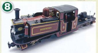
With all the screws removed and pipework separated, you can lift each end from the smokebox making sure you clear any pipework as you go. You can see one end has already been removed.
