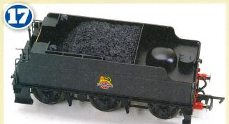
The tender body fits neatly back over the chassis as it did before, completing the sound installation. The tender speaker is an optional step in the sound fitting process but does enhance the decoder's audio performance.
