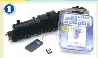
Dapol's new GWR'Mogul' has been designed with DCC and sound modellers in mind. It has a Next18 decoder socket in the smokebox on a pull-out PCB together with space for two speakers.
