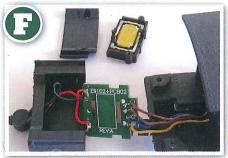
The supplied speaker plus the small PCB to which speaker and rear headlamp wires are attached can be seen. I made a note of the colour coding prior to the removal of all wires from the PCB.
