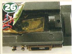
There isn't as much space inside the original design which means only a decoder and speaker can be fitted. The same Next18 adaptor board was used, wired up as per the diagram in Step 16. Kapton tape has been used to insulate the chassis area due to the tight confines of the space.
