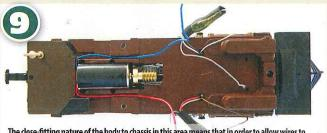
The close-fitting nature of the body to chassis in this area means that in order to allow wires to pass a channel must be made. I used a flat circular grinding disc in a minidrill to form a channel along the side of the backhead casting as shown. To retain as much structural integrity as possible, be careful not to remove too much material.
