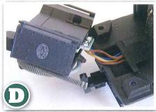
After removing the two retaining screws from below the rear of the footplate (see step A above) the coal bunker and footplate wiring cover plate can be lifted away.
