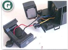
I soldered the speaker wires (brown) to the new larger speaker and joined the wires for the rear headlamp (red and black), insulating them with shrink wrap tubing. The speaker was insulated at the rear with Kapton tape. The bunker was refitted to the footplate with the speaker part way into the space created with a portion onto the centre of the footplate.
