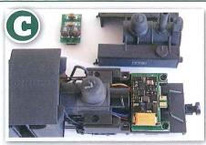
A push fit of the specially produced Zimo MX659N18 sound decoder is all the installation required. At this point the model can be reassembled and put into service using the factory fitted speaker. The following steps show how to fit an optional larger speaker.
