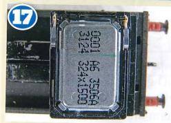
I reattached the speaker to its endosure using cyano (super) glue. The distortion in this extreme dose up makes it look as if the speaker is too big to fit, but
