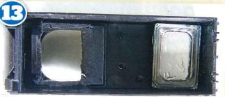
The 10mm x 15mm cube speaker, shown here without its enclosure, fits transversely below the tender top.
