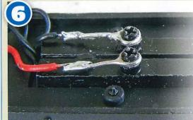
The wire used for the eyelets takes solder readily whilst the screws hold them tightly against the chassis halves. This arrangement provides good electrical continuity for the decoder to access track power. Note the fixing 'pip', the chassis internal side rails and the central raised area.
