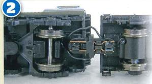
detail shows how the track power is connected locomotive and tender with brass strips. The black wires are from the decoder socket to the
