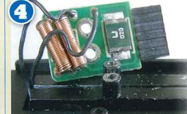
detach the (black) motor wires ready to solder to the decoder. The supporting towers should be shortened to about 2mm high with a fine file. Be careful not to remove too much as there needs to be enough thread remaining for the screws to tighten correctly.
