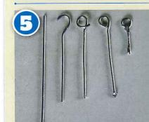
I made some evelets from scrap capacitor new connections for track power. the five stages of final of which was soldered for
