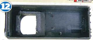
Most of the lower portion of the bunker was removed using a burr bit in a minidrill. A lip was left at the front and rear to support the metal coal load. An alternative would be to create a false floor from plastic sheet and cover it with crushed coal.
