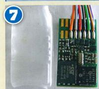
insulation, pictured left, was removed from the MX648 reduce the overall thickness. This by itself would not invalidate the warranty if reinsulated before use.
