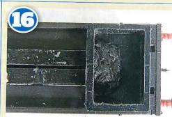
I carefully split the endosure from the speaker then fitted the endosure to the chassis. Any gaps were sealed with black mastic to create an airtight speaker endosure - essential for best
