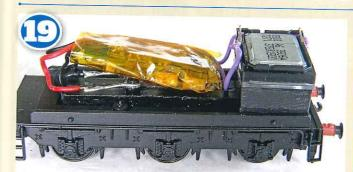
The decoder is wrapped in Kapton tape for insulation in this view showing the general disposition of components before reassembly. I also added some insulation to the tops of the screws and the eyelets for safety.
