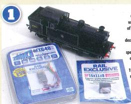
Oxford Rail's 'N7' 0-6-2T isn't blessed with a huge amount of internal space, but there is room for a decoder in the bunker. Finding space for a speaker was a greater challenge and even this small 15mm x 11mm cube speaker needed reducing in height to fit.
