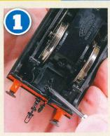
The process starts by turning the locomotive upside down to find the body fixing screws. The front screw is located above the front coupling mount which we had already removed from this model.
