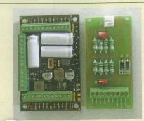
Zimo's flagship MX699KV large scale sound decoder (left of picture) is compared with the locomotive PCB which has now been removed from the model.
