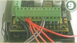
The black track wires and the red track wires from each bogie are joined together and connected to the appropriate screw terminals on the decoder. Similarly, the grey pair and the orange pair were connected together at the decoder. Unfortunately, this caused the wheels of one bogie to run in the opposite direct to those on the other on this example.
