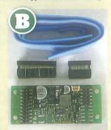
The MX696S with cable has the advantage of being self-contained, but the wires will need to be joined to the model's wiring by soldering or screw terminal blocks.
