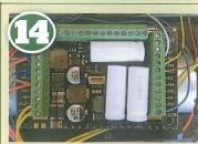
LEDs and the roof fan each have their own connection to the decoder. This allows more prototypical use of lighting possible with DCC operations
