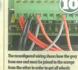
from one end must be joined to the orange from the other in order to get all wheels turning in the same direction. The actual direction depends on which motor output each pair is connected to. Incorrect direction can be reversed by using a CV29 value change, but it is easy to rectify in the wiring at this stage.
