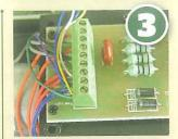
In close up, the wires to the headcode LEDs can be identified as yellow, white and blue. These and the JSP plug should be released to allow the body to be put aside for safety.
