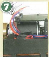
This support can be seen in its central position above the twin horizontally mounted motors. There is no need to lengthen any wires if the decoder is located here, though some may need uncoiling to nsure a stress-free connection.
