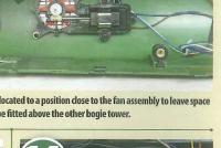
fan's operating speed I decided to retain it. The final wiring of the decoder shows that each pair of I released the screws holding this board and relocated it to a position next to the roof fan, fixing it with double-sided tape. The input wires from the board were connected to the common positive and FA3. The sound project
