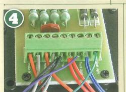
With the body mounted component connections removed, the track and motor connections can be seen more dearly.
