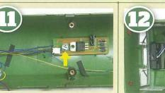
The operating radiator fan is controlled by this PCB. iometer (arrowed) is a convenient way to adjust the speed of the fan so this board was retained for its functionality.
