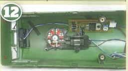
It was, however, relocated to a position close to the fan assembly to leave space for the speaker to be fitted above the other bogie tower.
