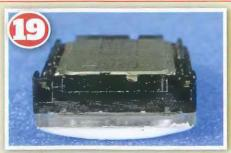
The speaker was prepared by removing its endosure and replacing it with a sized flat styrene sheet fixed with cyano adhesive. The styrene was filed to match the arched shape of the roof.
