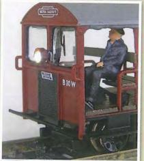
With the driver on board, the front lamp was illuminated and brightness adjusted with CV60 on the MX648.
