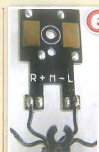
I disconnected the inner pair of wires labelled M+ and M- and tested them with a DMM and 12V power to confirm that they were the motor wires.
