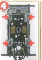
The slots for the bearings have tight dearances and each bearing must be precisely aligned before it can be pushed home.
