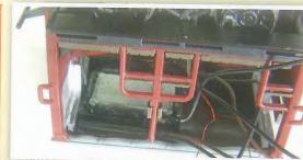
The modified speaker was fixed centrally in a longitudinal orientation, allowing wires from the chassis to pass either side on
