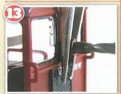
I held each lamp with tweezers whilst producing the required void for the LEDs with a 2.0mm drill, also in a pin vice. This stops the lamp body twisting and snapping from the cab front.
