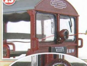
This shot shows the wires passing through the lamp and central pillar. An indication of the depth can also be made out by the dark inner rim of the modified lamp.
