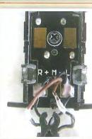
Viewed from above, the four added wires can be seen in the upper part of the chassis ready to be fed through the body to the decoder.
