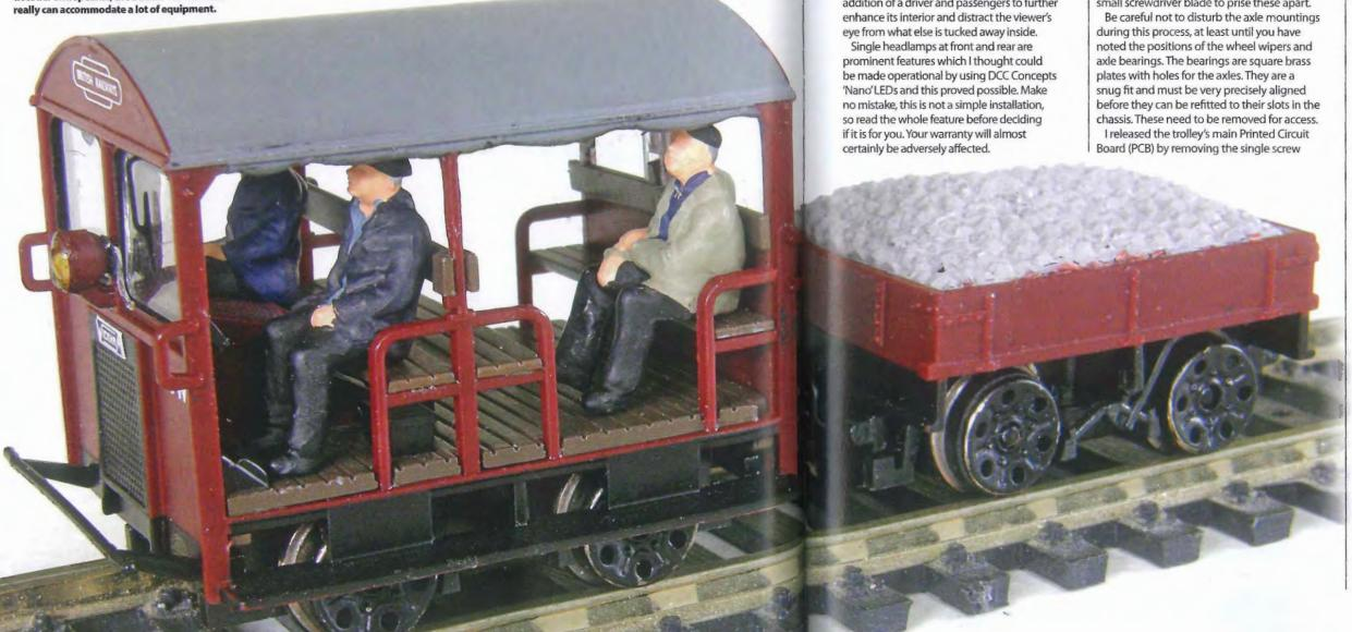
mouldings. To prepare them for LED installation, I marked the centres of each lamp with a bradawl prior to drilling through each lamp and continuing through the body, using a 0.4mm drill in a pin vice. This serves to pass the wires from the NANO LEDs to the inside of the body and to provide a guide for the 2mm drill I used to create a cavity in the body of each lamp.
