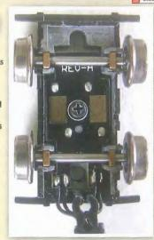
axle bearing arrangements. The incomplete circle of the front of the drawbar can be seen detached from the peg on the chassis.
