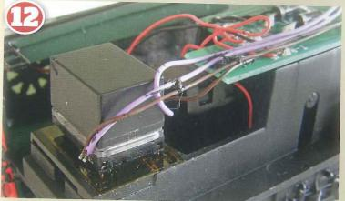
The purple speaker wires from the decoder were soldered to the connections on one speaker. Additional (brown) wires were also attached to link the other speaker in parallel and in phase. I routed these wires above the locomotive PCB to avoid contact with the flywheels, cardan shafts and bogie towers.
