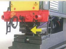
bodyis into position. he very strong magnet in the speaker attracts the three link coupling arrowed) which prevents the body from sliding into its correct position, so take recautions to avoid this.
