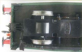
I found that access to fit the end caps was dramatically improved by temporarily removing the bogie side mouldings. Here one side is fitted and the other removed, illustrating the two push fit fixings on each side. This completes reassembly of the locomotive ready for it to
