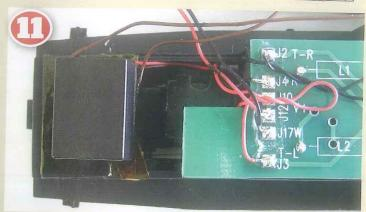
In the first variation I installed a Zimo cube speaker at each end fixed in place with black mastic. Blu Tack would work too — each providing a semi-permanent adhesive.
