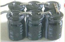
to the twin installation eated a 166,666 µF pacitor pack by connecting six 2.7 volt 1F supercapacitors n series. This raises the oltage to 16.2v, perfect for e dedicated 16v regulated upply from the MX645
