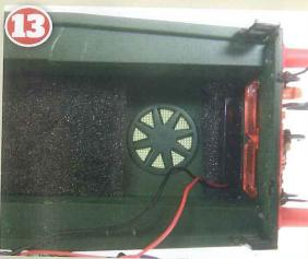
I cut off a portion of the foam inside each engine room to expose the radiator fan grille and create clearance for each speaker.
