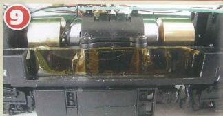
The MX645R will be installed in this space at the lower side of the cab. I insulated the chassis in places where solder pads or components may make contact in use.
