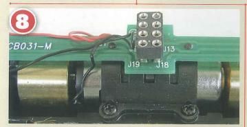
With the body removed, the central motor and 8-pin connector can be seen clearly. Here the blanking plug has been removed.
