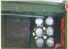
The pack fits snugly in the space available. but to ensure it doesn't move around I used a little mastic to hold
